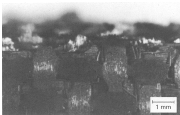
Figure 4 Surface of fracture in the SiC/SiC material.
